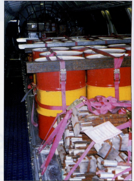
With the passenger seats removed, this 737 aircraft transports camp gear, fuel and survey monuments from Yellowknife to Rankin Inlet.
